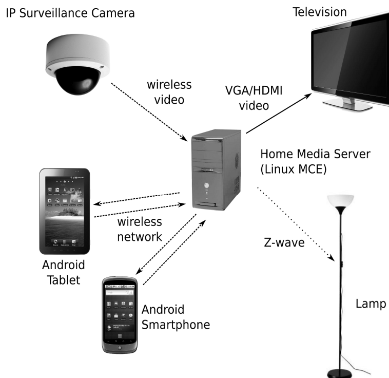
FIGURE 1: Overall system architecture of the Virtual Teratak
