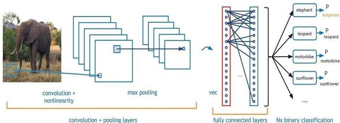
FIGURE 2: Deep model architecture (CNN).
