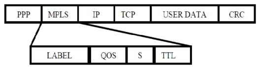
Figure 3: Showing the MPLS header Format
