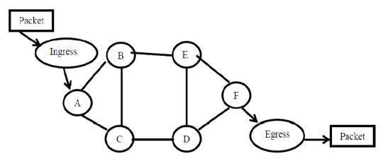
Figure 1.1: showing working of MPLS subnet with Egress and Ingress router attached
