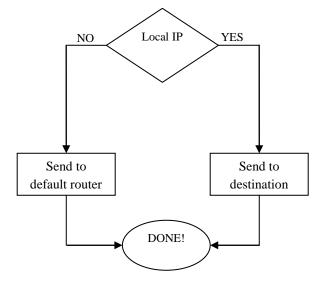
FIGURE5.1.b: Transmission process after apply the Hypothesis
