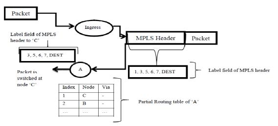
Figure 2: Showing the add MPLS header by ingress router and how to move from A to C.
