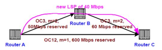
Figure 4: Constraint Based Routing
