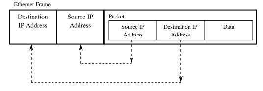
FIGURE 5.2.b: New Proposed Ethernet frame
