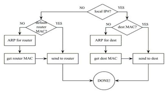
FIGURE5.1.a: Current Procedure for Transmission one Frame process
