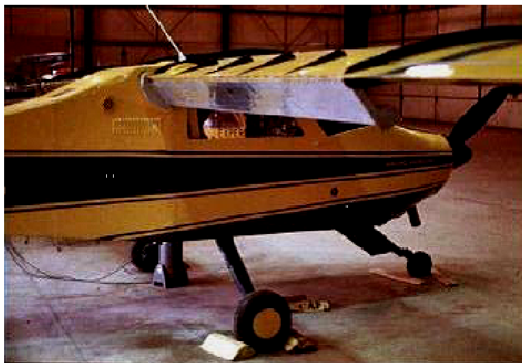
FIGURE 3. Trailing Edge Coandă Surface Extended From WVU Flight Demonstrator [30].
