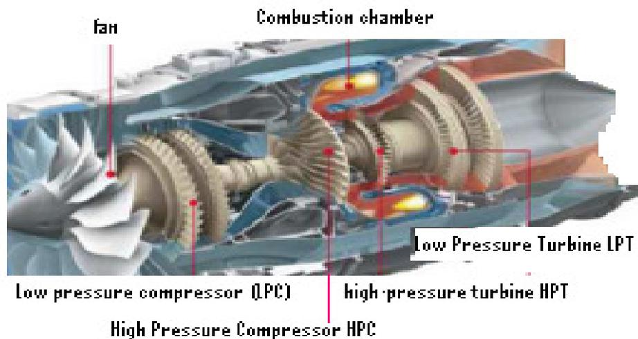
FIGURE 1: Turbojet Components.
