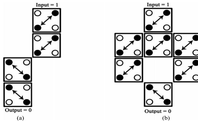
FIGURE 3: QCA Inverters: (a) Corner Inverter, (b) Robust Inverter.
