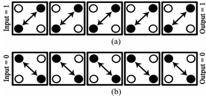
FIGURE 2: QCA wires: transmitting (a) “1” and (b) “0”.
