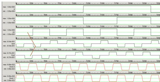
FIGURE 9: New QCA Full Adder Simulation Results.
