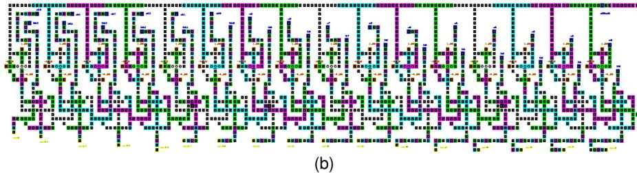
FIGURE 16: (a) QCA Layout of 8-bit Adder-subtractor, (b) QCA Layout of 16-bit Adder-subtractor.
