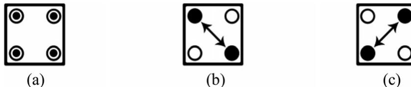
**FIGURE 1:** QCA cell: (a) empty cell, (b) polarization -1, (c) polarization +1.
