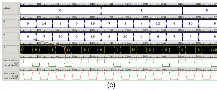
FIGURE 15: 4bit Adder-subtractor: (a) Block Diagram, (b) QCA Layout, (c) Simulation Results.
