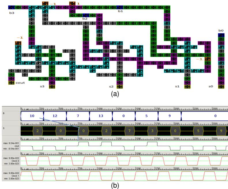
FIGURE 12: Binary to BCD Converter: (a) QCA Layout, (b) Simulation Results.
