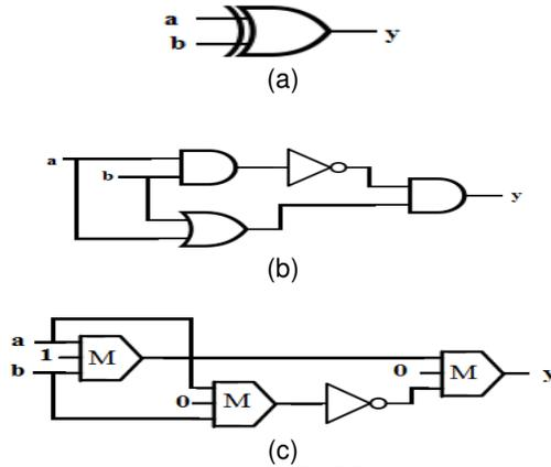
**FIGURE 13:** XOR gate: (a) logic symbol, (b) AND, OR realization, (c) majority gate realization.
