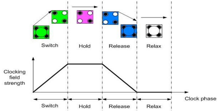
FIGURE 5: Four clock phases in QCA.
