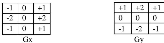
**FIGURE 1:** Masks used by Sobel Operator
