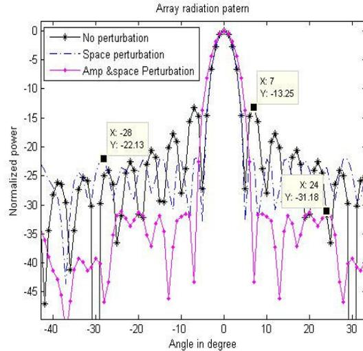
**Figure 1:** Results for 16 elements linear antenna array
