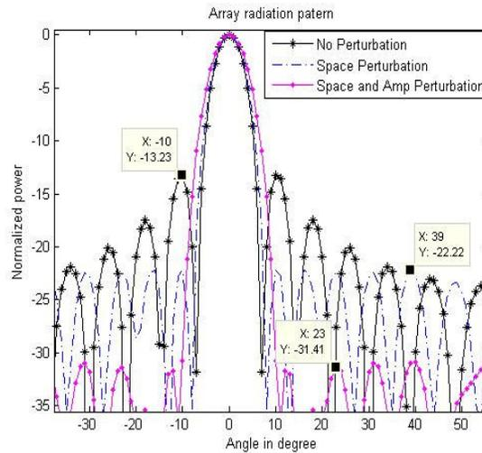
**Figure 2:** Results for 24 elements linear antenna array
