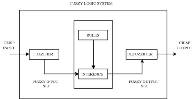
**FIGURE 4:** The structure of a fuzzy logic system
