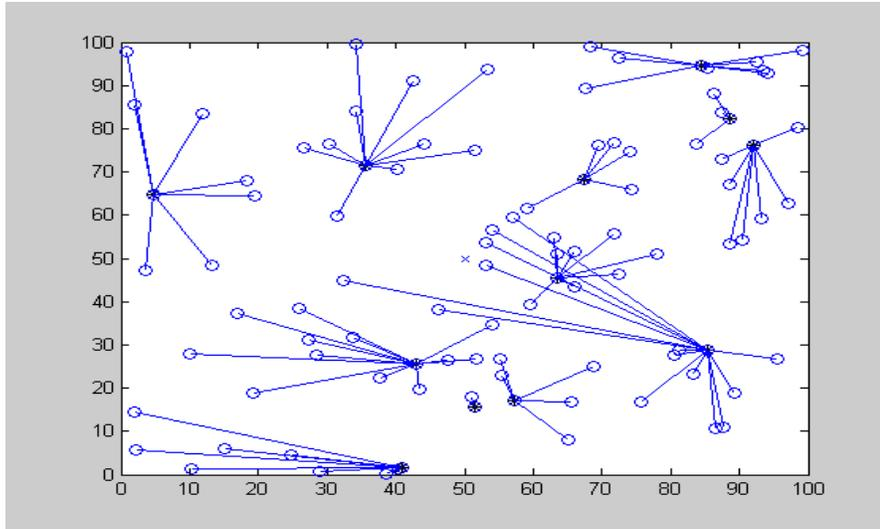
**FIGURE 3 (a):** 100-node random sensor network for round1
