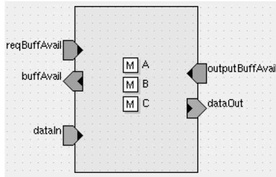
**Figure 10:** MLD Implementation of the OutputBuffer Class.
