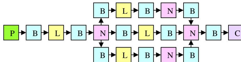
**Figure 4:** NoC Model for Interaction Between One Producer Process and One Consumer Process.
