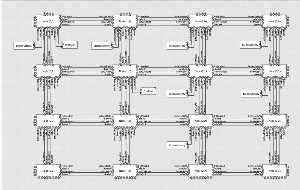
**Figure 11:** MLD Implementation of 4x4 Mesh NoC.
