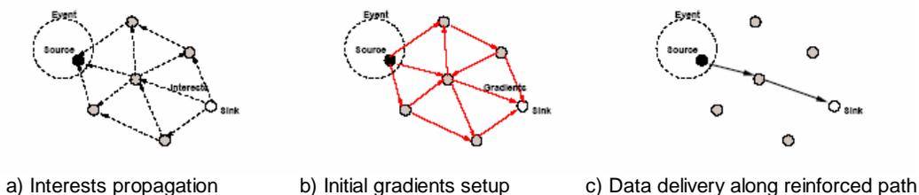
Figure 1: A simple schematic for directed Diffusion [1]
