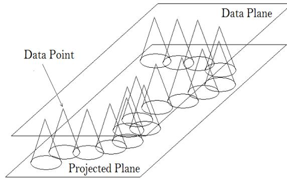
**FIGURE 7:** Concept of IDS (Ink Drop Spread)[24]
