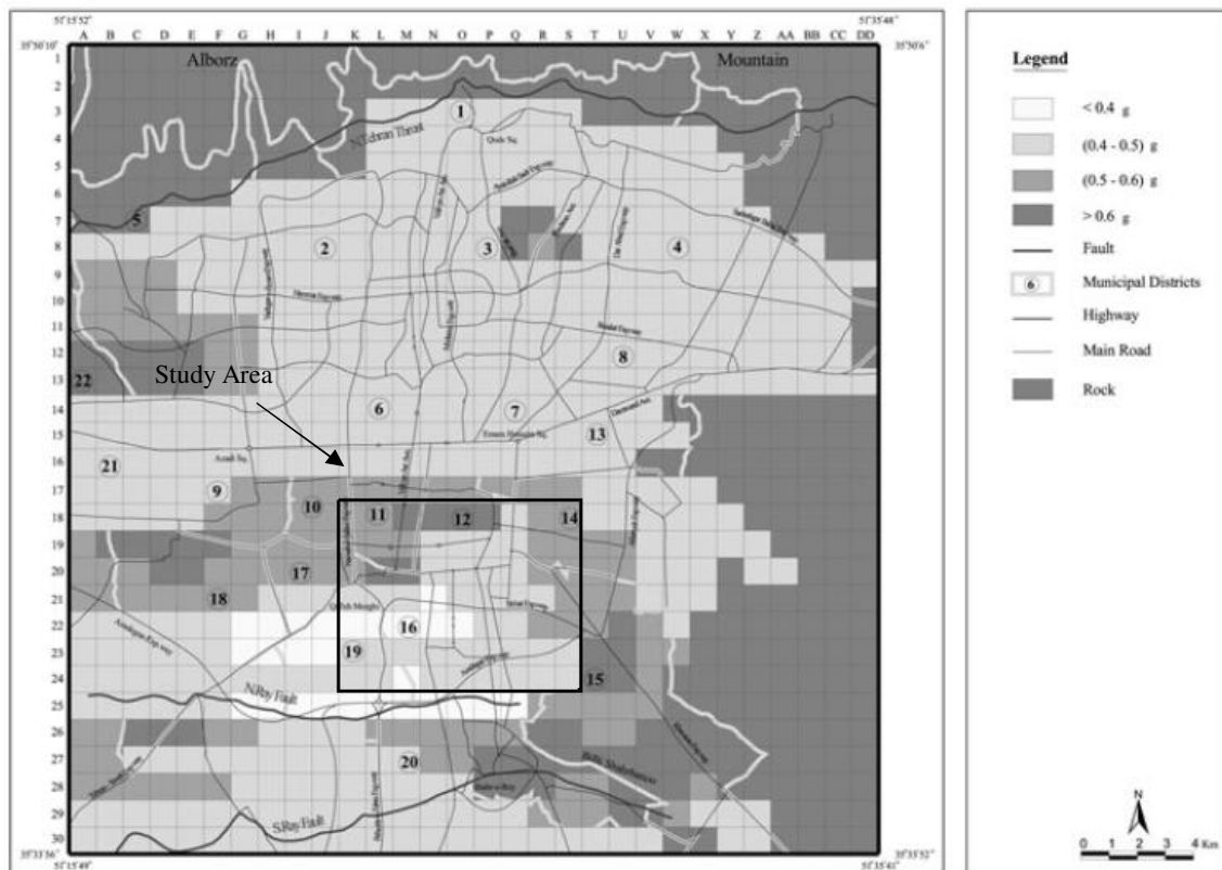
FIGURE 1: The study area and PGA distribution throughout Tehran for an earthquake corresponding to 475 year return period [24].
