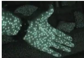
FIGURE 3: Real IR light dots that IR Emitter sends [33].
