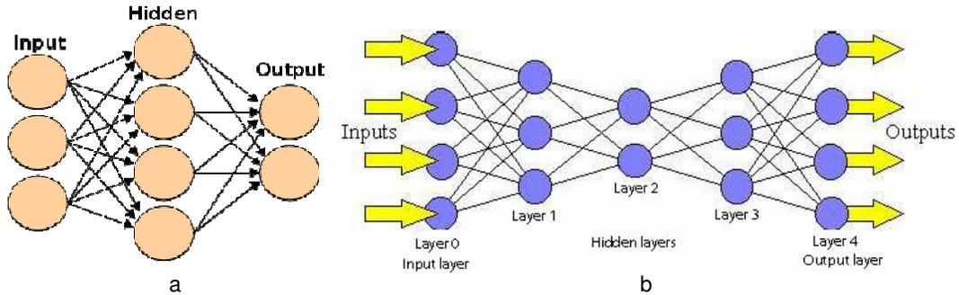
**FIGURE 4:** Feed forward Networks types. (a) Simple Feed forward Networks. (b) Multiplayer Feed forward Networks. (From internet image gallery)
