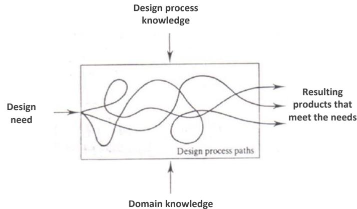
**FIGURE 1:** Knowledge used in the design process [1].
