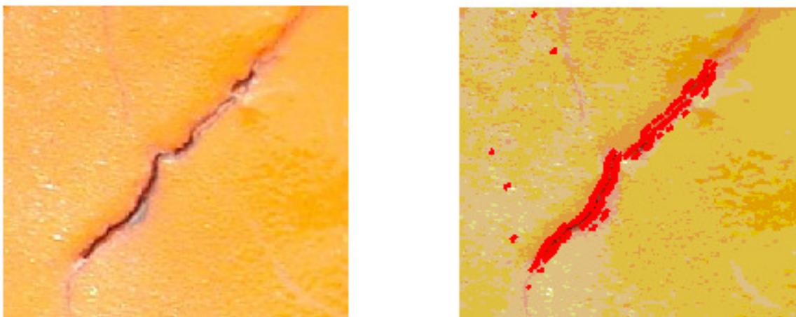
**FIGURE 4:** Marking of Crack by Gabor Filter
