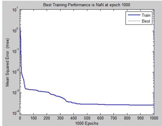
**FIGURE 8:** Mean Squared Error for Scaled Conjugate Gradient.
