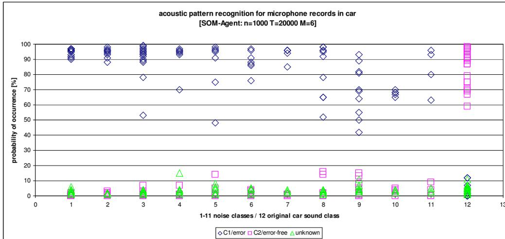
**Figure 5:** SOM2-Agent statistic: A calculated probability of occurrence for 129 measurements, SOM with 1000 neurons and 6 parameters is used. Legend defines whether the analyzed measurements are assessed as “error”, “error-free” or “unknown” condition.
