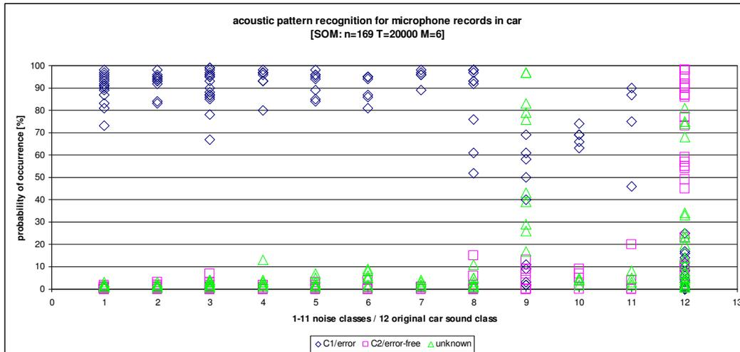
**Figure 4:** SOM1-Agent statistic: A calculated probability of occurrence for 129 measurements, SOM with 169 neurons and 6 parameters is used. Legend defines whether the analyzed measurements are assessed as “error”, “error-free” or “unknown” condition.
