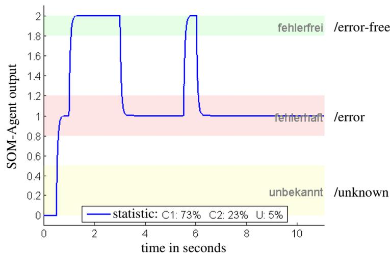
**FIGURE 2:** Autonomous detection of noticeable acoustic changes in car interior. The SOM-Agent characteristic curve (blue) toggles between three sound classes “error-free”, “error” and “unknown” sound, e.g. if output value is “1” the microphone recording was made in a car with damaged or worn-out parts.
