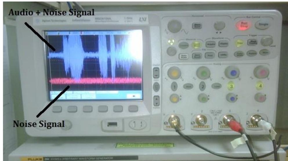
FIGURE 14: Acquired Data Through Microphones.
