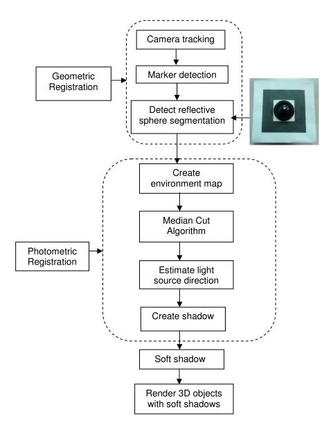
FIGURE 1: Frameworks of System Prototype.
