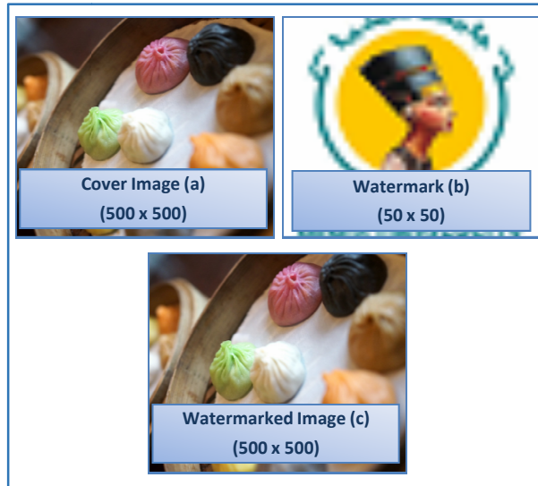
FIGURE 4.1: Embedding a, b using Modified MSLDIP Watermarking to output the watermarked image c.
