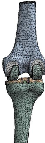
**FIGURE 5:** Meshed assembly of implant system configuration
