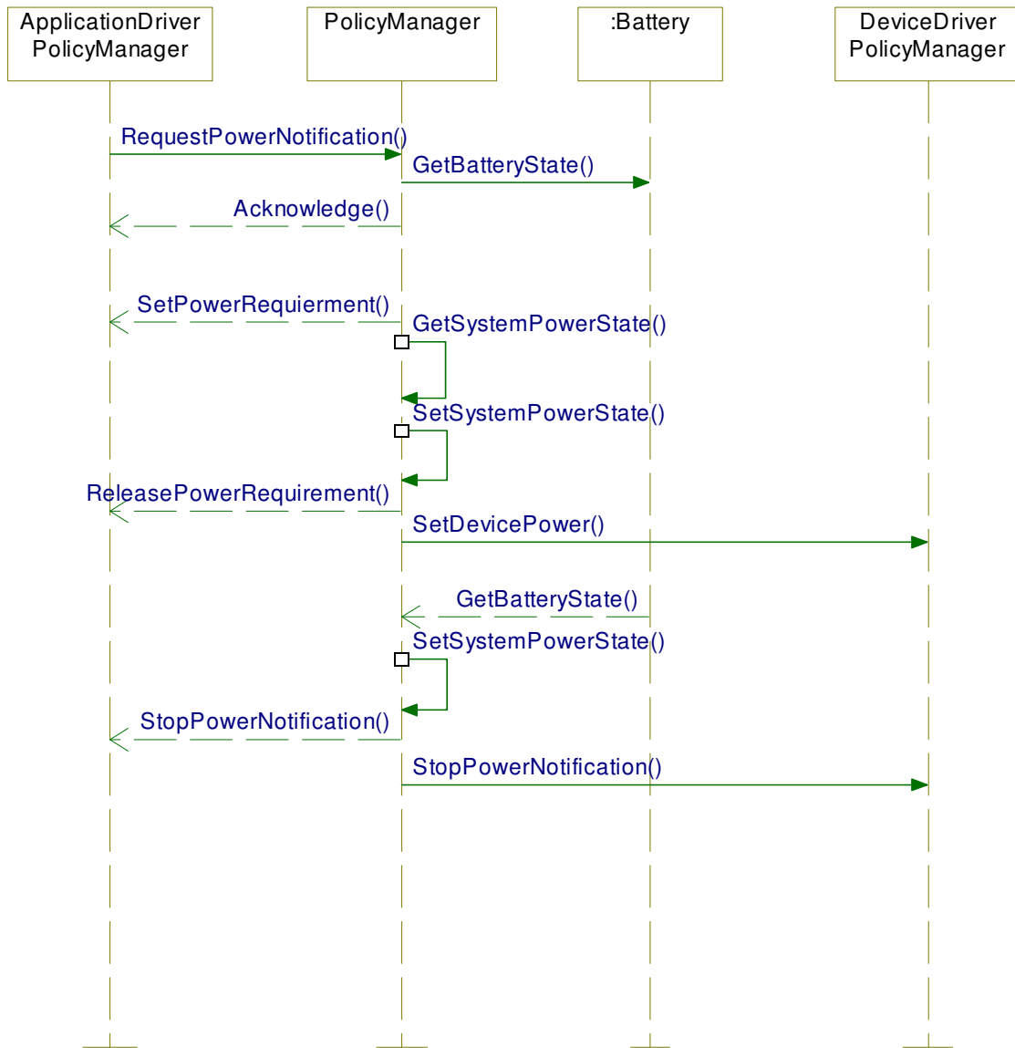
Figure 10: Sequence Diagram of Application Driver Power Manager Interaction with Power Manager
