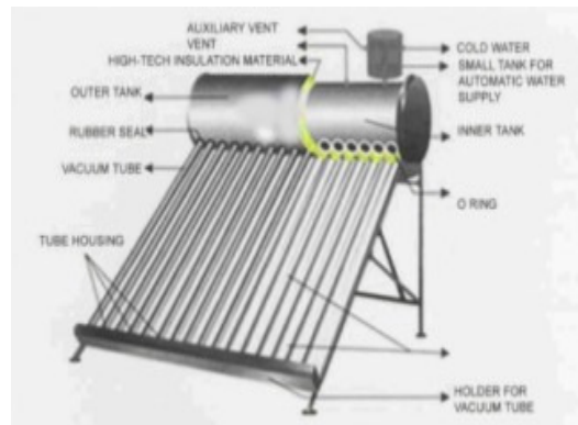
FIGURE 2: Evacuated tube solar water heater
