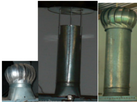
FIGURE 2: Three devices under test: (from left to right) turbine ventilator, straight column, and the combined turbine-column device.
