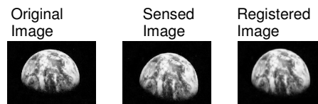
FIGURE 8 Registration of sensed images differ by rotation, scaling and translation from original image.
