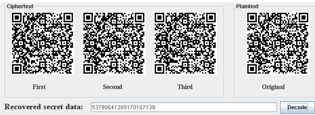
FIGURE 6: Recovery of secret message from three barcode tags using (3, 3)-threshold.
