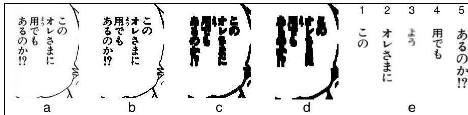
FIGURE 5: Sample of Text Extraction Process (a) Original balloon text image; (b) Threshold; (c) Morphology-Erosion filter; (d) Morphology-Opening filter; (e) Extracted blob from original image
