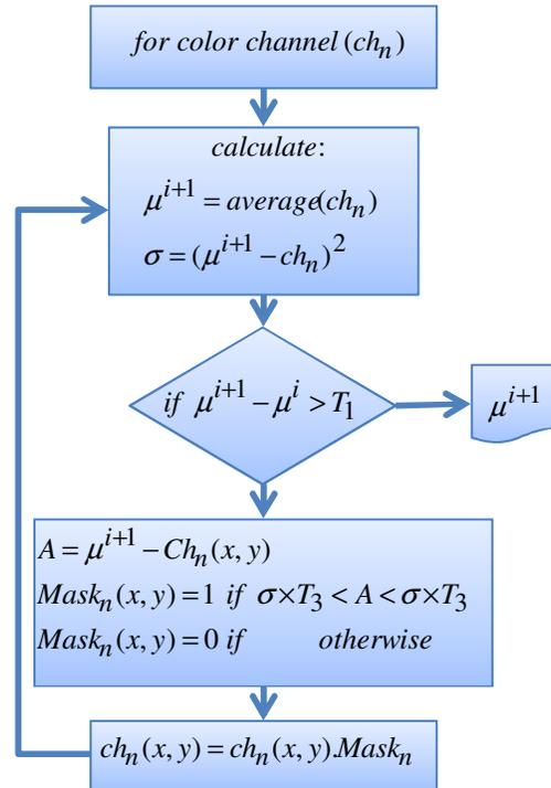
FIGURE 4: Different steps of color segmentation process
