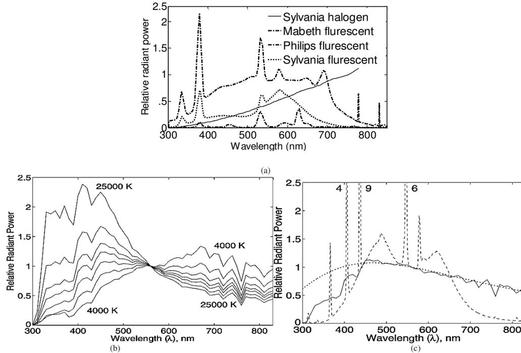
**FIGURE 2:** Different light sources with their SPDs. (a) SPDs for three different fluorescent lamps compared to SPD of halogen bulb [23]. (b) Daylight SPDs at different hours of day, normalized at 560nm. (c) Spectra of different light sources all with a CCT of 6200K and normalized at  $\lambda = 560$  nm [24].
