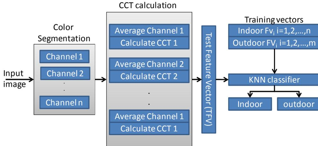
**FIGURE 3:** Block Diagram of the proposed method for indoor-outdoor classification
