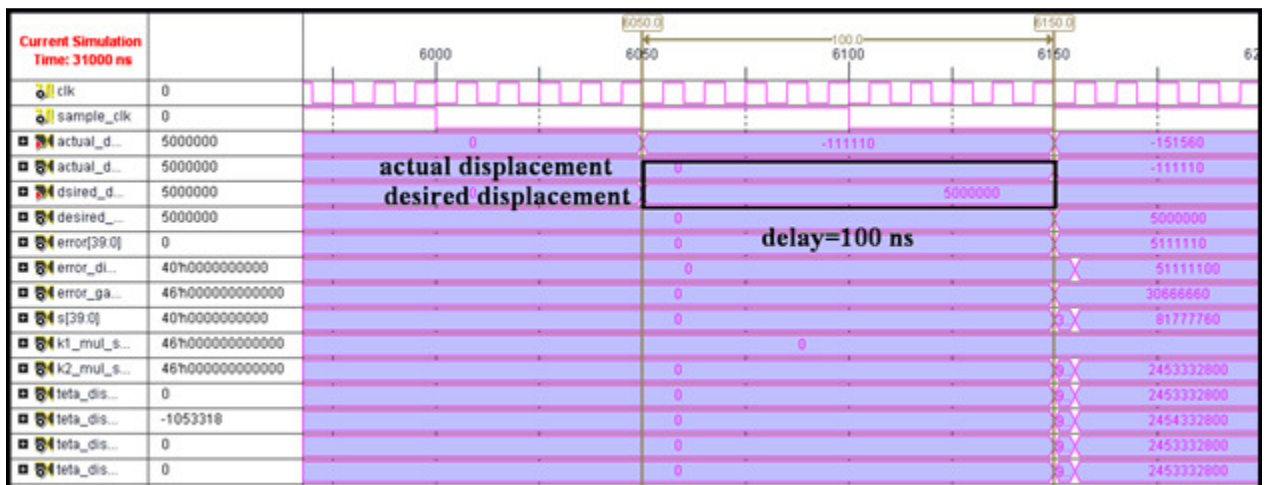
FIGURE 14 : The delay time in PD-SMC between desired displacement and actual displacement
