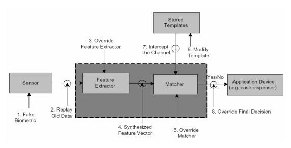
(Fig1. Vulnerable in biometric system)
