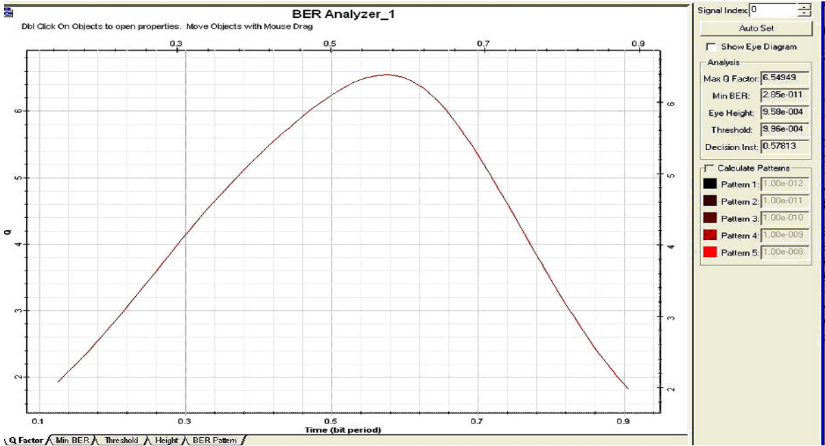
FIGURE 11 Q factor v/s Bit period for NRZ system at bandwidth of 1566nm at the distance of 240KM
