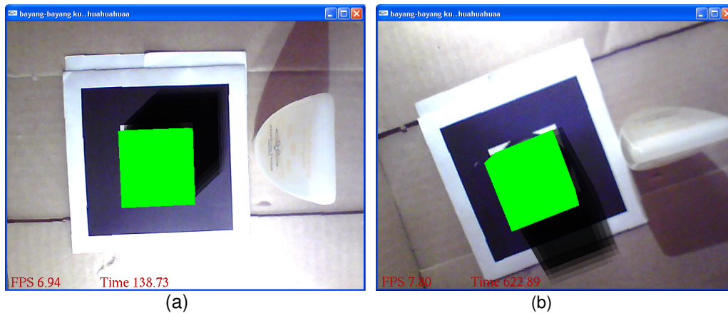
FIGURE 6: Shadow of Computer Generated Object Based on Real Light Position.
