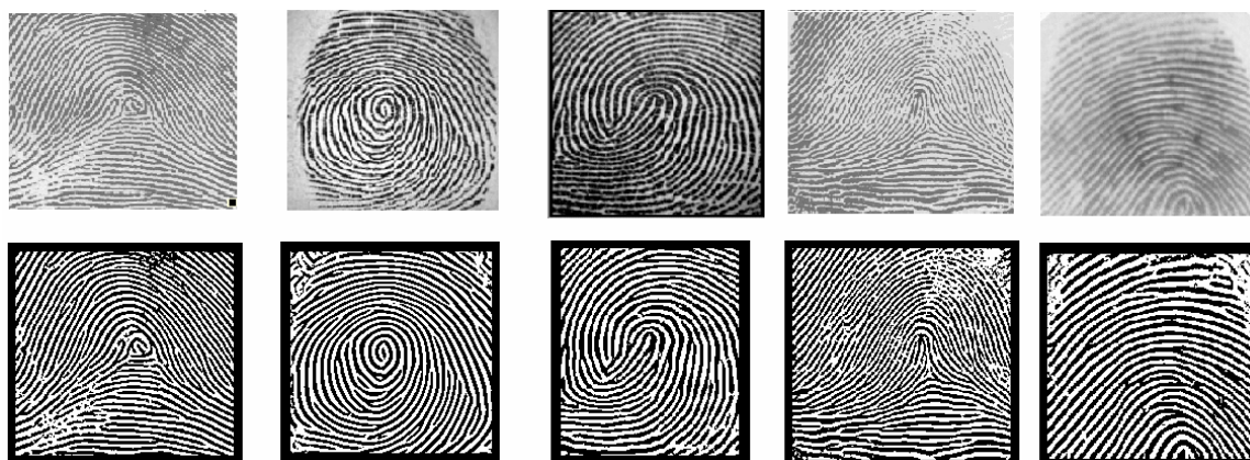
Figure 4 : The first row shows the original images. The second shows the enhanced and binarized images correspondingly.
