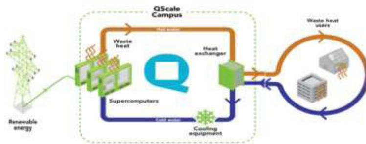
FIGURE 2: Recovery of waste heat from a Qscale Campus. Source: opencompute.org.
