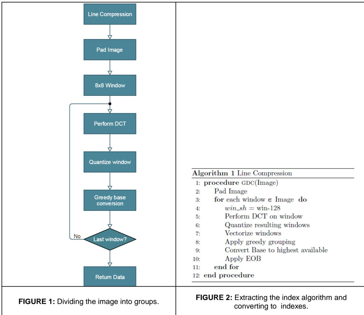
The first figure is the diagram of the function which divides the block into small groups and then the groups into the corresponding indexes. The second one is its pseudo code.
