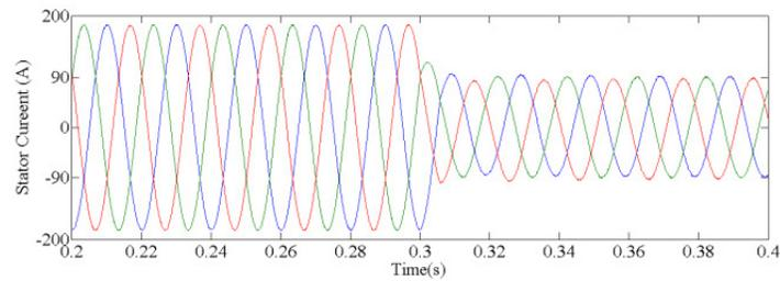
**FIGURE 20:** Three phase stator current
