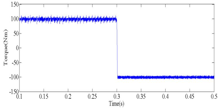
**FIGURE 13:** Output torque of DTC based on IMC
