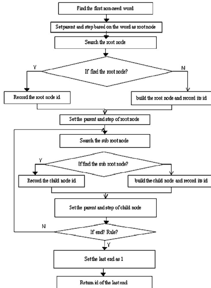
FIGURE 11: The Flow Chart of Matching Algorithm.
