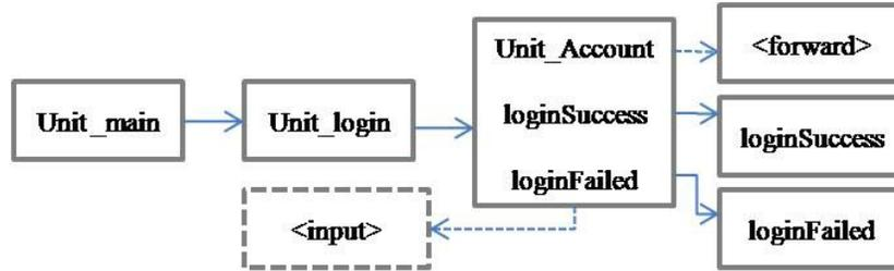
FIGURE 3: The MVC structure of login Model
