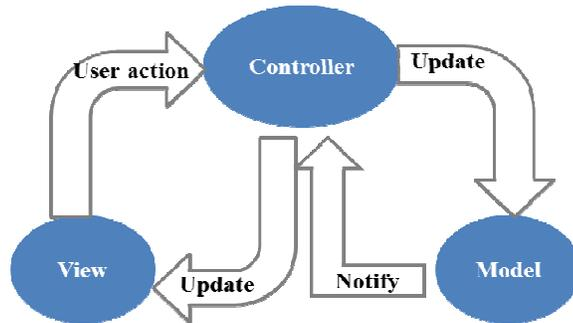
FIGURE 1: The Interactions Between M, V and C.
