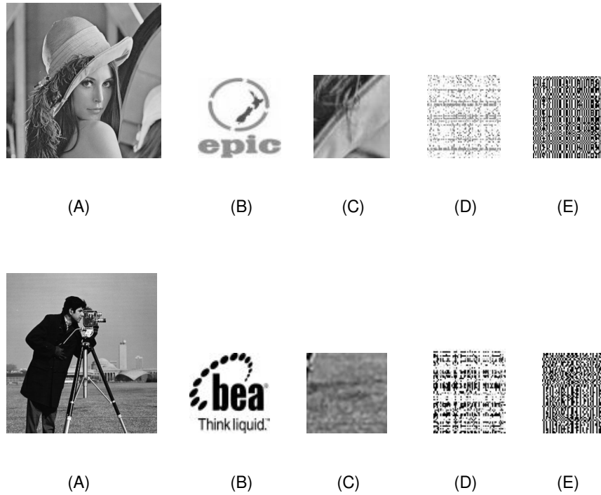
FIGURE: 2 Intermediate results of PSCV construction A - Primary Image(512 * 512) , B - Patent Image(64 * 64) , C -Sub primary Image(64 * 64) D - Shuffled Patent Image (IS) (64 * 64) , E - Projected Image(64 * 64).
