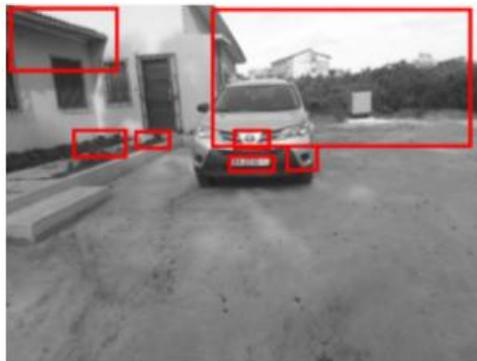
**FIGURE 1:** Outcome of the detection and the extraction of plates zones.
