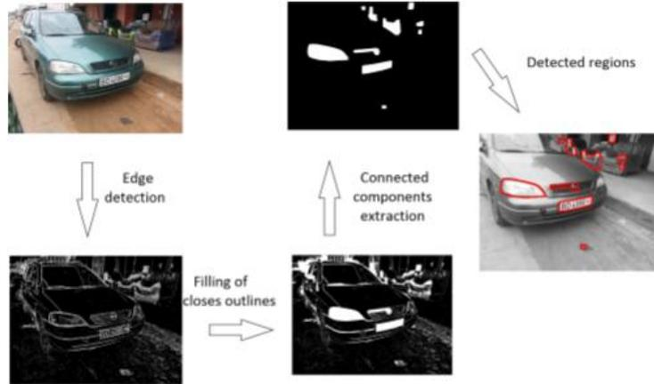
**FIGURE 2:** Detection of plate by detection of outlines
