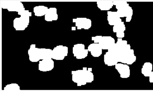
Fig 2.9 Global threshold using Otsu's method
