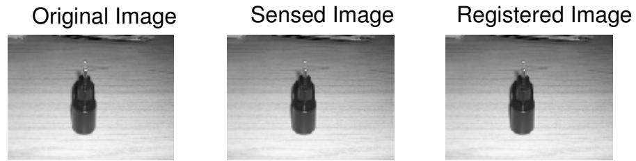
FIGURE 5: Sensed image is translated by dx= 34 , dy=-34
