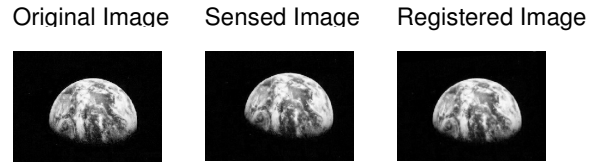
FIGURE 7 Registration of sensed images differ by rotation, scaling and translation from original image.
