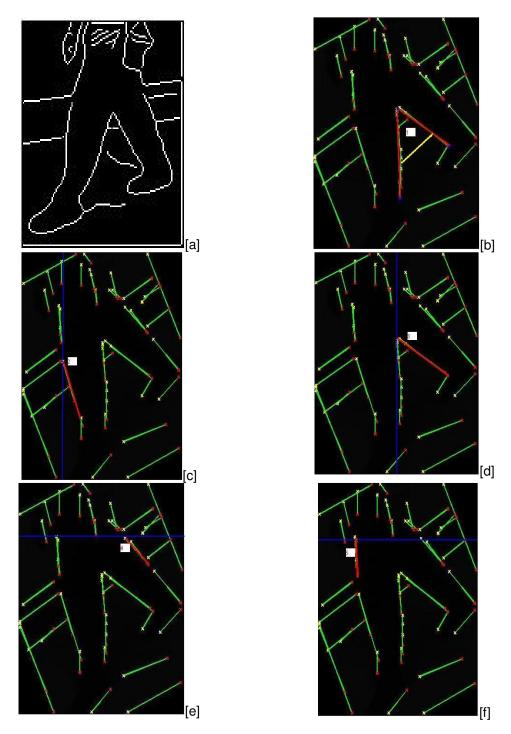
**FIGURE 4**: The Hough transformed image indicating different parameters. [a] edge detected image [b] distance between legs [c] right knee angle [d] left knee angle [e] left thigh angle [f] right thigh angle.
