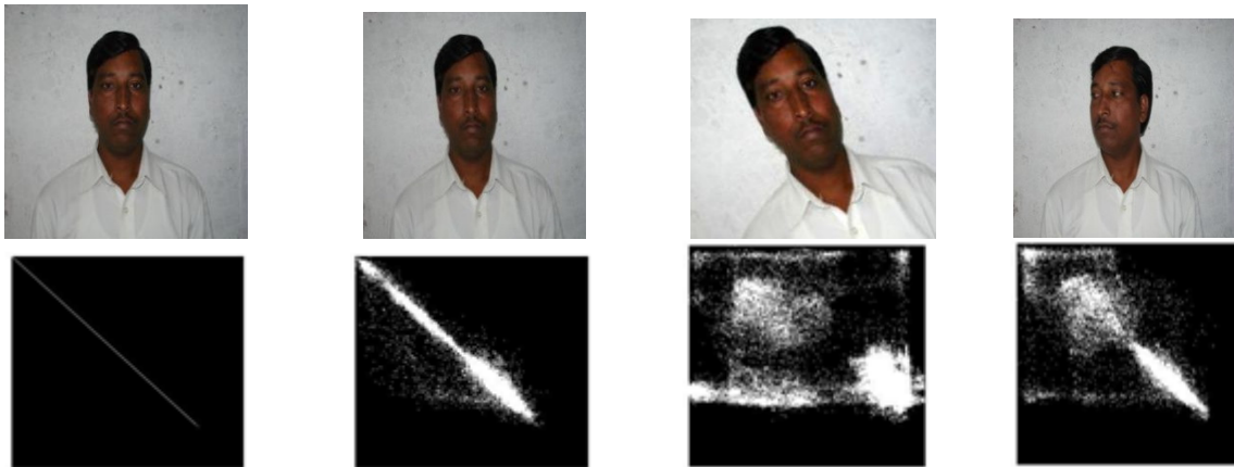
a b c d e f g h FIGURE 8: ( a ) Subject. ( b ) subject rotated by 5 0 .(c) Subject rotated by 20 0 .(d) Subject with rotated neck. (e) Joint histogram a Vs a. (f) Joint histogram a Vs b. (g) Joint histogram a Vs c. (h) Joint histogram a Vs d .
