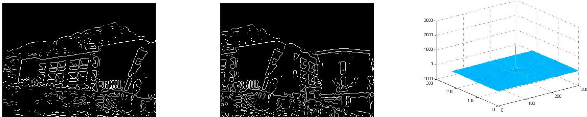
FIGURE 13: (a) Edges extracted from SCOE-1. (b) Edges extracted from SCOE-2. (c) cross power spectrum for SCOE 1 & SCOE 2 in frequency domain.
