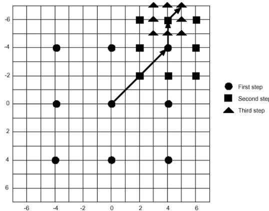
**FIGURE 2:** Three Step Search Procedure. (Motion Vector is (5,7))
