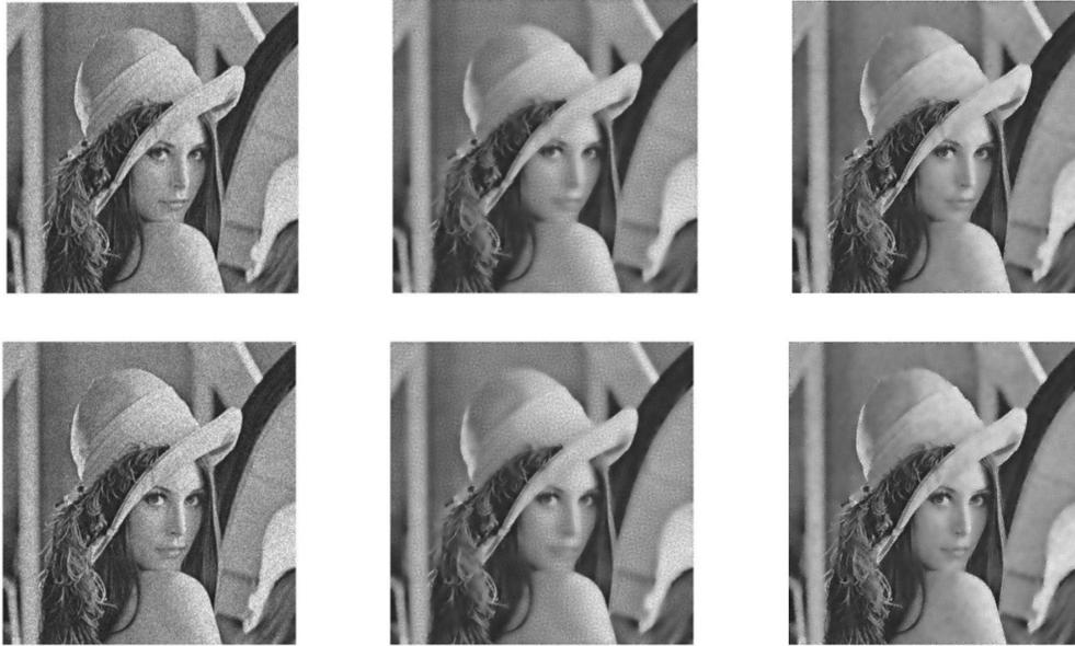
**FIGURE 3:** Kuan filter results with different NLOOK values. Gaussian and Uniform noise distributions are used in the top and bottom rows respectively. Each row shows (from left to right): the noisy image, the Kuan filtered image using NLOOK=ENL and the corresponding Kuan filtered image using NLK\_AD with  $A=0.65$ . An  $11 \times 11$  window with images of size  $256 \times 256$  are used.
