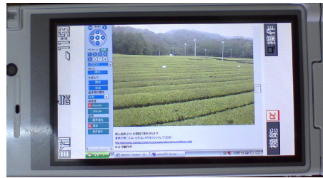
(c) Camera image data (natural colored image and near infrared image are monitored with mobile phone)
