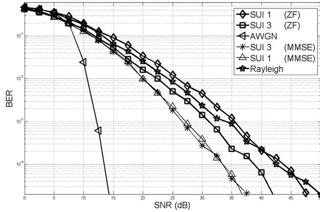
FIGURE 3: Performance Simulation (ZF and MMSE)
