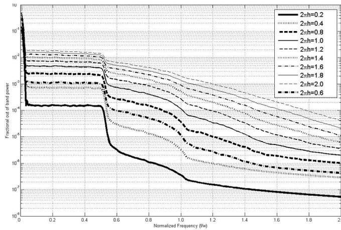
FIGURE 5: Fractional out of band power Simulation (Modulation index effect)
