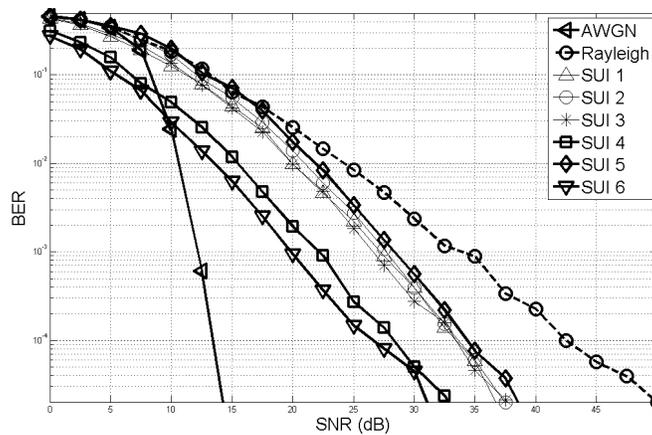
**FIGURE 2:** OFDM-CPM Performance Simulation (M=4, N=256, MMSE)
