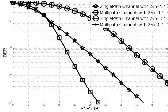
FIGURE 4: Performance Simulation (Modulation index effect)
