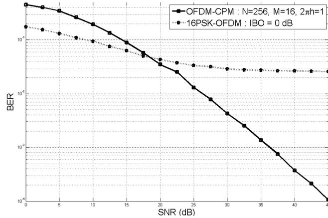
FIGURE 6: Performance Simulation (OFDM-CPM and 16PSK-OFDM)
