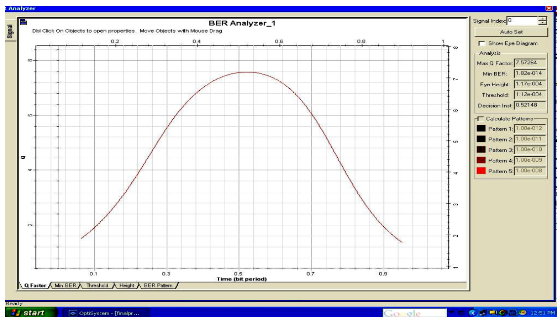
FIGURE 10 Q factor v/s Bit period for NRZ system at bandwidth of 1566nm at the distance of 120 KM.
